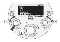
function, or that you tune manually are displayed as you turn the **TUNE** control. You can change the order in which the stations are displayed. See the "DAB Display" and "Display Menu"
